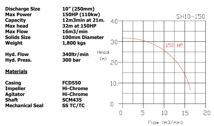
The main features of our heavy duty slurry pump is a heavy design of wear resistant casing and 28% HiCr impeller. Excellent combination of materials provides long term operation even in harsh abrasive slurries.
