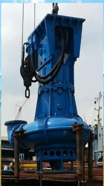
DISCHARGE SIZE 16 INCH (400MM).HIGH PRESSURE MECHANICAL SEAL.DESIGNED FOR HEAVY SAND SLURRIES.
