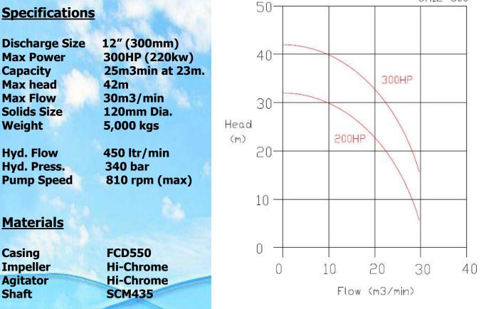
The main features of our heavy duty slurry pump is a heavy design of wear resistant casing and 28% HiCr impeller. Excellent combination of materials provides long term operation even in harsh abrasive slurries.
