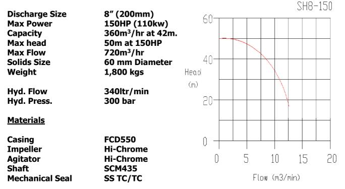
The main features of our heavy duty slurry pump is a heavy design of wear resistant casing and 28% HiCr impeller. Excellent combination of materials provides long term operation even in harsh abrasive slurries.
